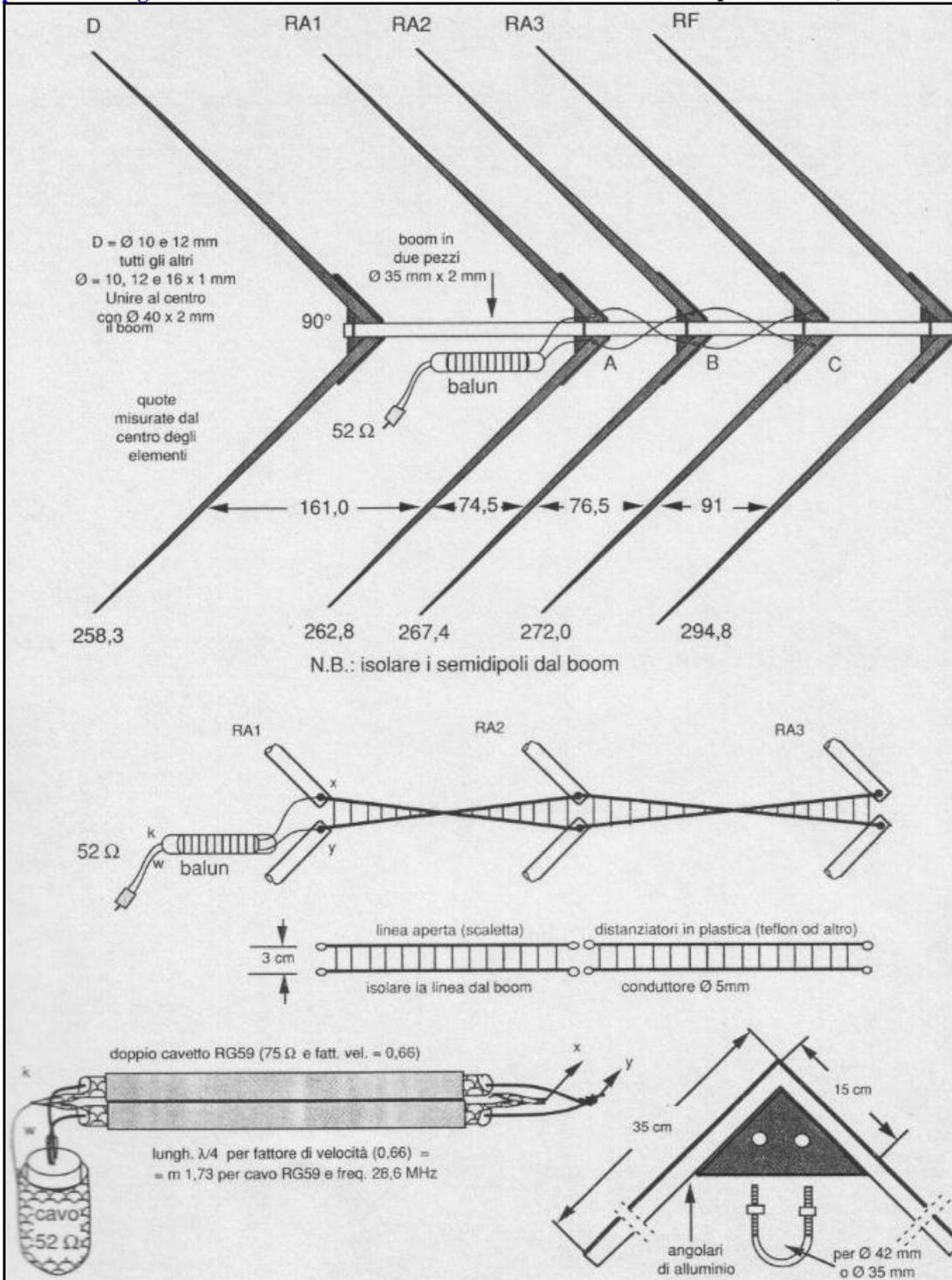
balun:10 turns made by double RG59 coax on a core made by 3 ferrite rods
